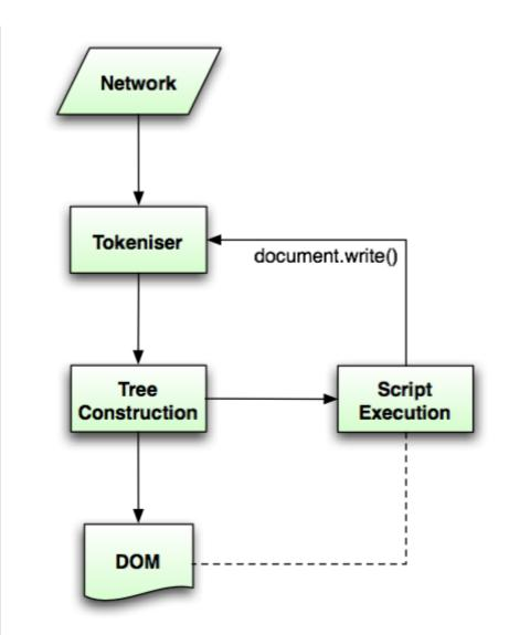
There is only one set of state for the tokeniser stage and the tree construction stage, but the tree construction stage is reentrant, meaning that while the tree construction stage is handling one token, the tokeniser might be resumed, causing further tokens to be emitted and processed before the first token's processing is complete.
